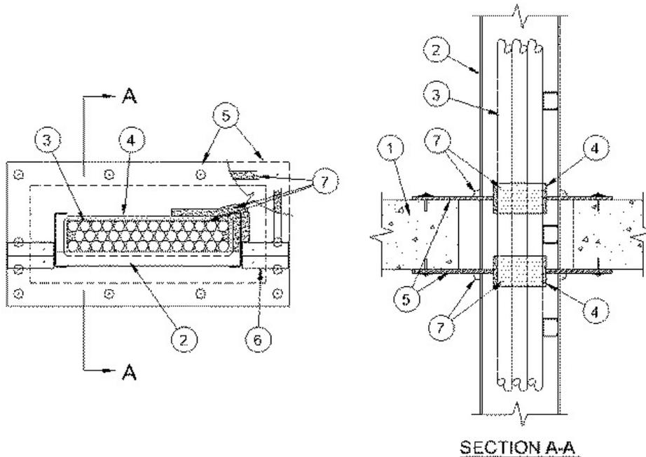
**1. Floor or Wall Assembly** — Min 4-1/2 in. (114 mm) thick lightweight or normal weight (100-150 pcf or 1600-2400 kg/m<sup>3</sup>) concrete. Wall may also be constructed of any UL Classified **Concrete Blocks\***. Max area of opening 900 sq in. with max dimension of 30 in.
