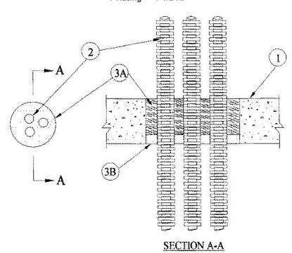
1. Floor or Wall Assembly — Min 4-1/2 in. thick reinforced lightweight or normal weight (100<u>150</u> pcf) concrete. Wall may also be constructed of any UL Classified **Concrete Blocks**\*. Max diam of opening is 4 in.
