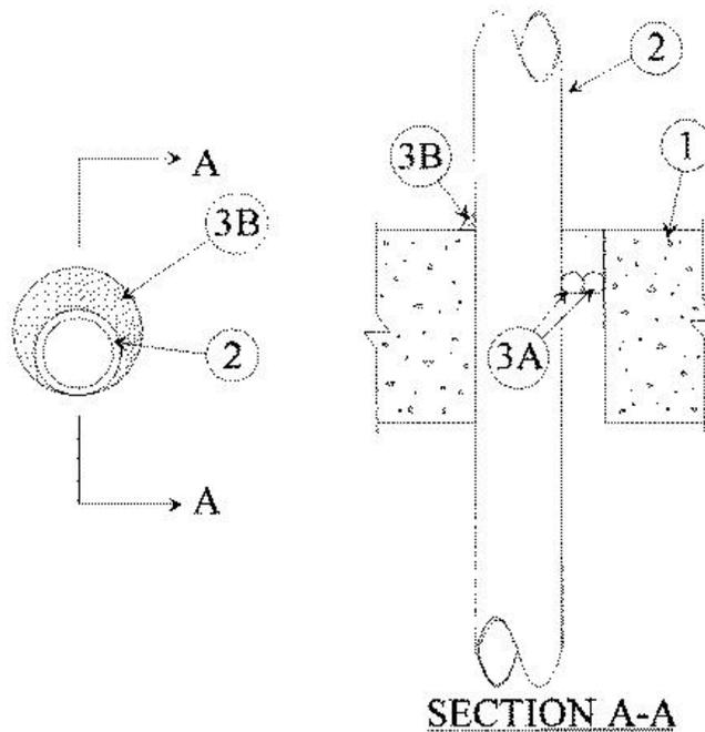
1. **Floor or Wall Assembly** — Min 4-1/2 in. thick reinforced lightweight or normal weight (100-150 pcf) concrete. Wall may also be constructed of any UL Classified **Concrete Blocks\***. Max diam of opening is 4 in. See **Concrete Blocks** (CAZT) category in the Fire Resistance Directory for names of manufacturers.
