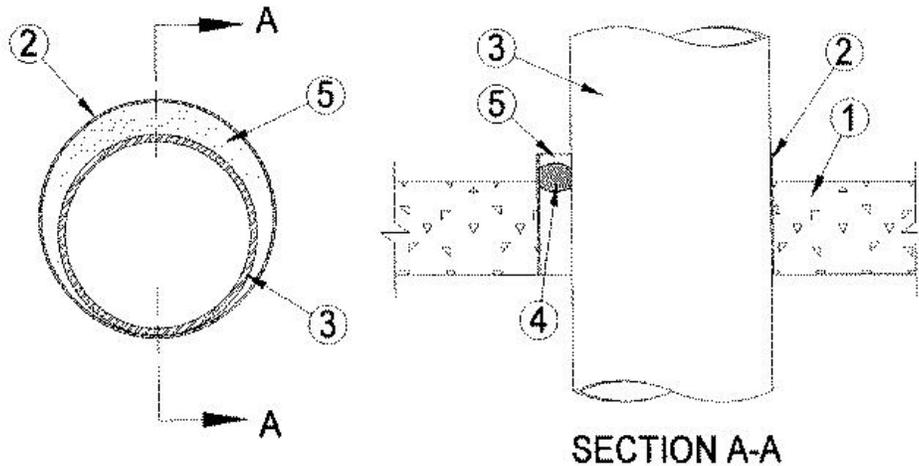
**1. Floor or Wall Assembly** — Min 4-1/2 in. (114 mm) thick reinforced lightweight or normal weight (100-150 pcf - 1600-2400 kg/m<sup>3</sup>) concrete. Wall may also be constructed of any UL Classified **Concrete Blocks**\*. Floor may also be constructed of any 6 in. (152 mm) thick UL Classified hollow-core Precast Concrete Units\*. See **Concrete Blocks** (CAZT) and **Precast Concrete Units** (CFTV) categories for names of manufacturers.
