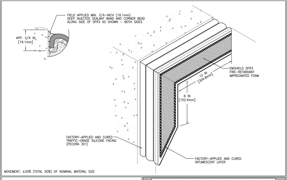
EMSEAL'S EMSHIELD DFR3 HAS BEEN TESTED IN ACCORDANCE WITH UL 2079 IN THE CONFIGURATION DEPICTED IN UL SYSTEM # FF-D-1090 . USE OF THIS MATERIAL IN DECK ASSEMBLY CONFIGURATIONS OTHER THAN DEPICTED IN UL SYSTEM # FF-D-1090 WILL NOT ENCUMBER OR LOWER THE RESISTANCE OF THE DECK BUT IS DONE SO AT THE DESIGNERS' DISCRETION AND RESPONSIBILITY FOR DESIGN OF A FIRE RATED DECK ASSEMBLY THAT MEETS APPLICABLE STANDARDS FOR THE PROJECT.
