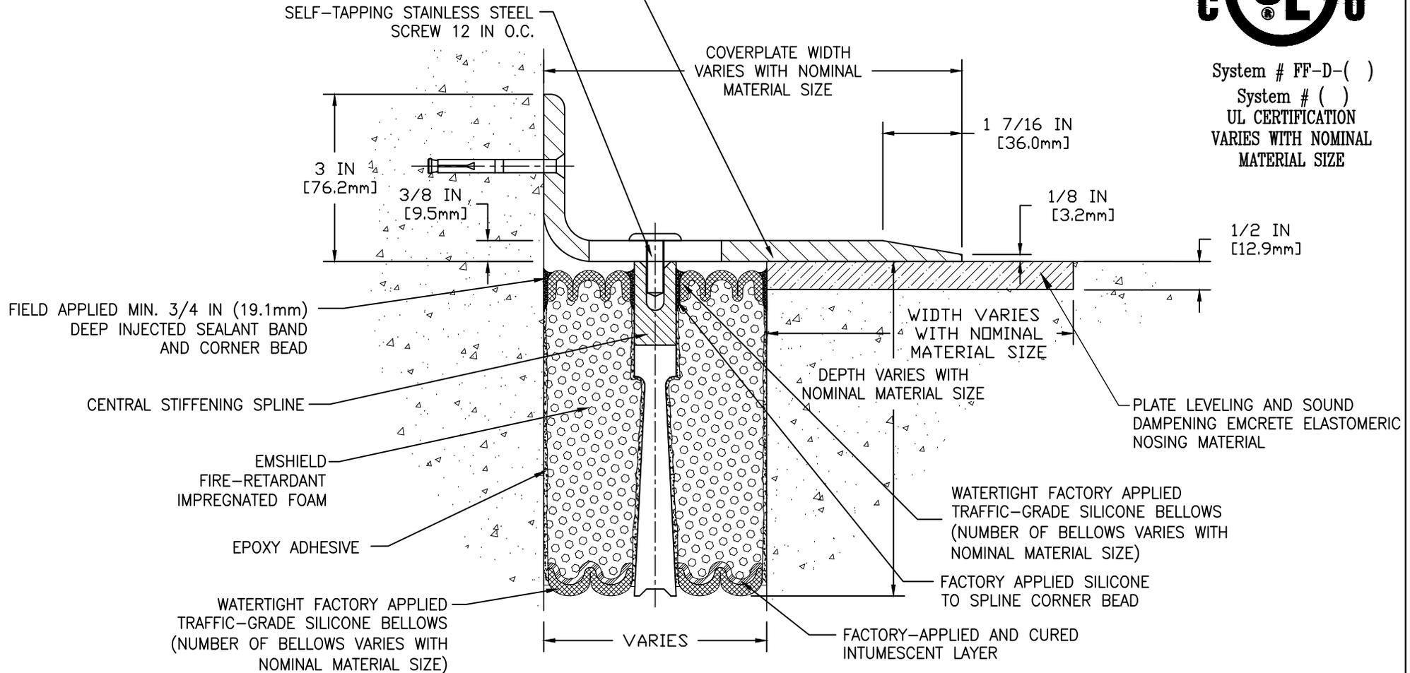
NOTE: 3/8 IN (9.5mm) COVERPLATES FOR VEHICLE AND PEDESTRIAN-TRAFFIC USE
