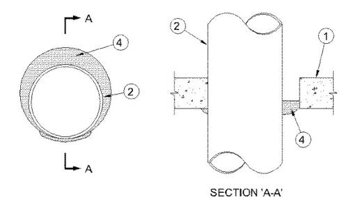
1. **Floor or Wall Assembly** — Min 4-1/2 in. (114 mm) thick reinforced light weight or normal weight (100<u>150</u> pcf OR 1600-2400 kg/m³) concrete. Wall may also be constructed of any UL Classified**Concrete Blocks\***. Floor may also be constructed of any 6 in. (152 mm) thick UL Classified hollow core **Precast Concrete Units**. Max diam of opening is 9-5/8 in. (244 mm). When precast concrete units are used the max diam of opening is 7 in. (178 mm).
