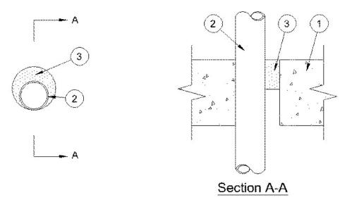
System tested with a pressure differential of 50 Pa between the exposed and the unexposed surfaces with the higher pressure on the exposed side.
