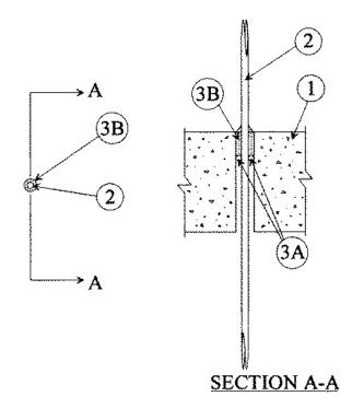
1. Floor or Wall Assembly — Min 4-1/2 in. thick reinforced lightweight or normal weight (100<u>150</u> pcf) concrete. Wall may also be constructed of any UL Classified **Concrete Blocks**<sup>\*</sup>. Max diam of opening is 1/2 in. See **Concrete Blocks** (CAZT) category in the Fire Resistance Directory for names of manufacturers.
