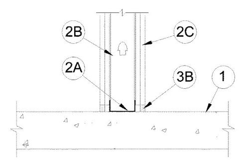
1. Floor Assembly — Min 4-1/2 in. (114 mm) thick reinforced lightweight or normal weight (100<u>150</u> pcf or 1600-2400 kg/m<sup>3</sup>) structural concrete. Floor may also be constructed of any min 6 in. (152 mm) thick UL Classified hollow-core **Precast Concrete Units**\*.
