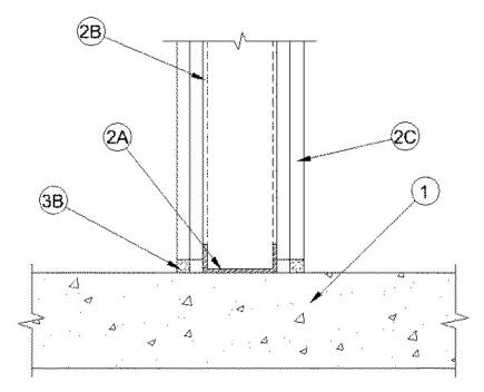
1. **Floor Assembly** — Min 4-1/2 in. (114 mm) thick reinforced lightweight or normal weight (100 <u>150</u> pcf or 1600-2400 kg/m<sup>3</sup>) structural concrete. Floor may also be constructed of any min 6 in. (152 mm) thick UL Classified hollow-core **Precast Concrete Units**\*
