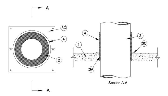
1. Floor or Wall Assembly — Min 4-1/2 in. (114 mm) thick reinforced lightweight or normal weight (100 $\frac{150}{100}$  pcf or 1600-2400 kg/m³) concrete. Wall may also be constructed of any UL Classified Concrete Blocks\*. Max area of opening is 13.75 ft (1.28 m²) with max dimensions of 44-1/2 in. (1.13 m).
