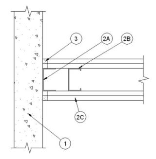
1. **Concrete Wall Assembly** — Min 4-1/2 in. (114 mm) thick reinforced lightweight or normal weight (100<u>150</u> pcf or 1600-2400 kg/m<sup>3</sup>) structural concrete. Wall may also be constructed of any UL Classified **Concrete Blocks**\*.
