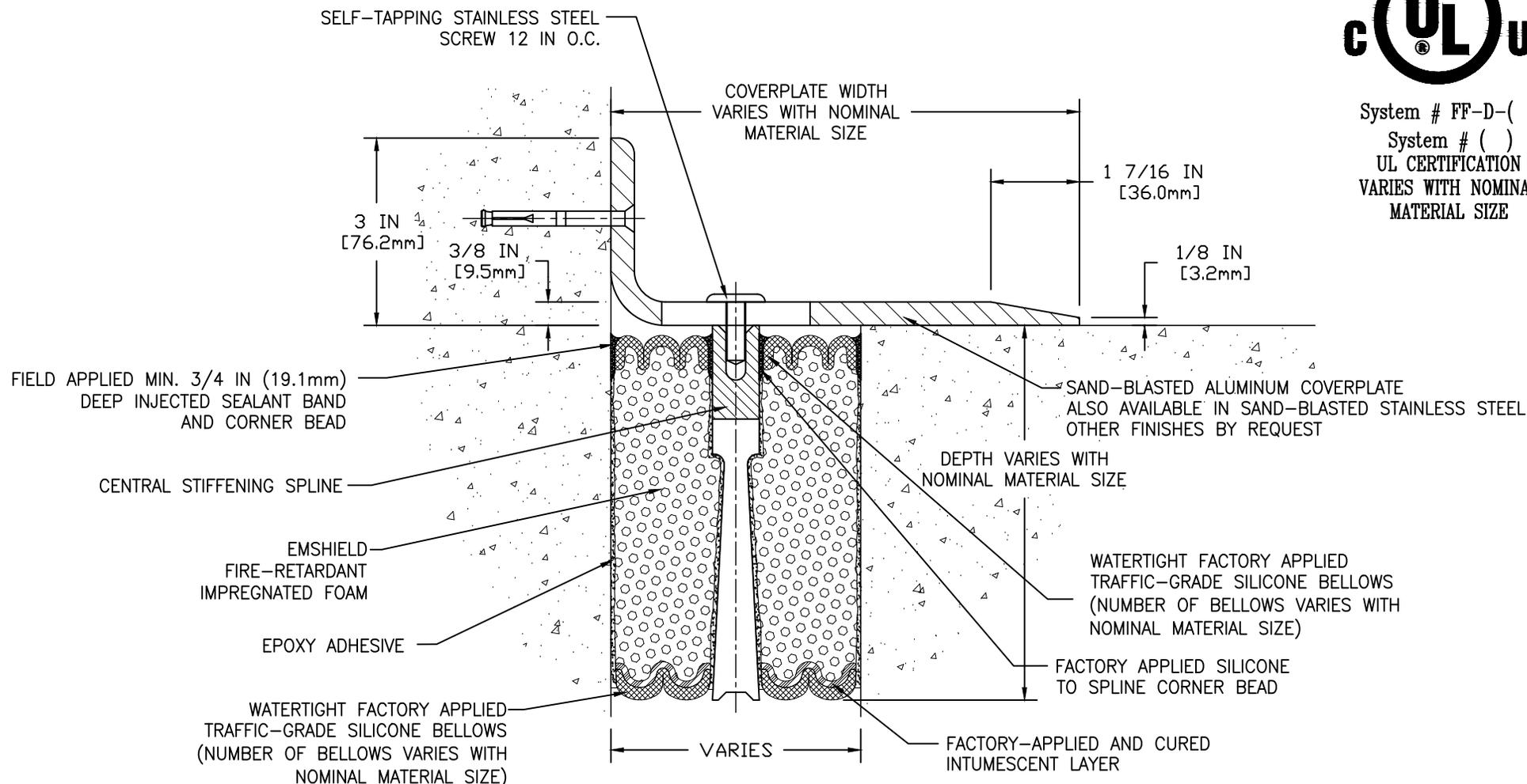
NOTE:  $\frac{3}{8}$  IN (9.5mm) COVERPLATES FOR VEHICLE AND PEDESTRIAN-TRAFFIC USE (FOR PEDESTRIAN-TRAFFIC ONLY, USE  $\frac{1}{4}$  IN (6.4mm) COVERPLATE)
