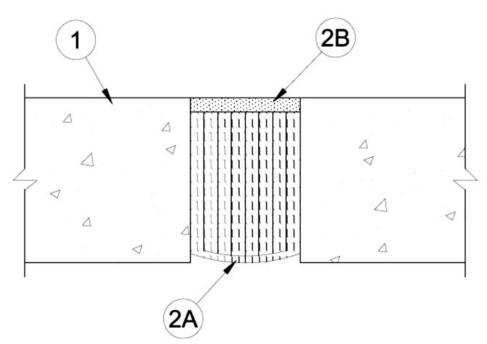
1. Floor Assembly — Min 6 in. (152 mm) thick reinforced lightweight or normal weight (100<u>150</u> pcf or 1600-2400 kg/m<sup>3</sup>) structural concrete.
