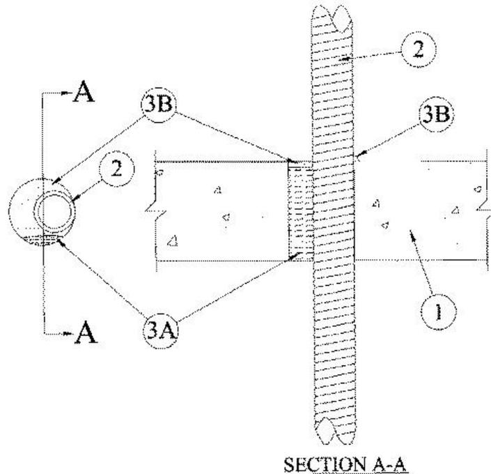
1. **Floor or Wall Assembly** — Min 4-1/2 in. thick reinforced lightweight or normal weight (100-150 pcf) concrete. Wall may also be constructed of any UL Classified **Concrete Blocks\***. Max diam of opening is 3 in.
