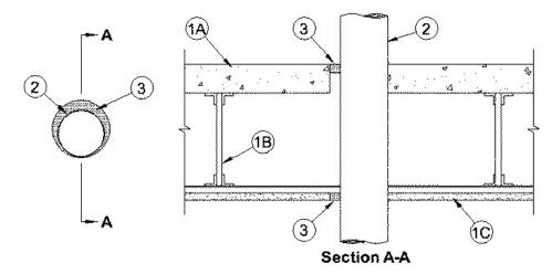
1. **Floor-Ceiling Assembly** — The 1 hr fire-rated concrete and steel joist Floor-Ceiling assembly shall be constructed of the materials and in the manner described in the individual G500 Series Design in the UL Fire Resistance Directory, as summarized below:
