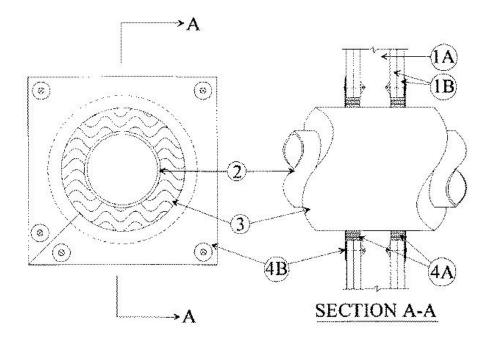
1. **Wall Assembly** — The fire-rated gypsum wallboard/stud wall assembly shall be constructed of the materials and in the manner specified in the individual U300 or U400 Series Wall and Partition Designs in the UL Fire Resistance Directory and shall include the following construction features:
