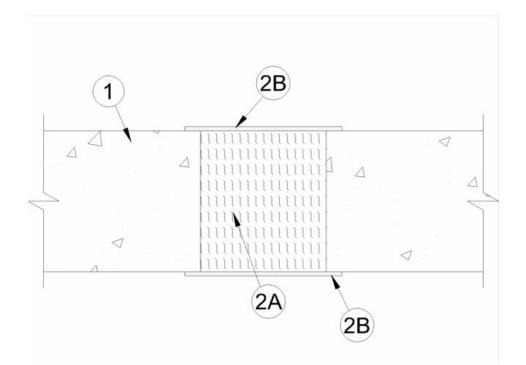
1. **Wall Assembly** — Min 4-1/2 in. (114 mm) thick reinforced lightweight or normal weight (100<u>150</u> pcf or 1600-2400 kg/m<sup>3</sup>) structural concrete. Wall may also be constructed of any UL Classified **Concrete Blocks**\*.
