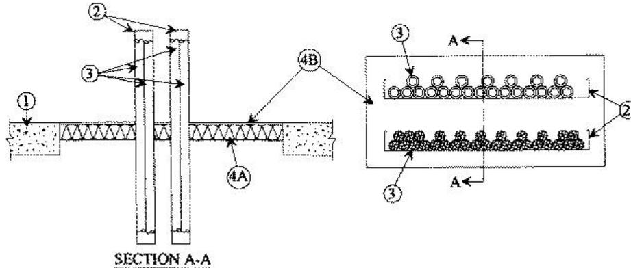
1. **Floor or Wall Assembly** — Min 4-1/2 in. thick reinforced lightweight or normal weight (100-150 pcf) concrete. Wall may also be constructed of any UL Classified **Concrete Blocks\***. Max area of opening is 960 sq in. with max dimension of 40 in. See **Concrete Blocks** (CAZT) category in the Fire Resistance Directory for names of manufacturers.
