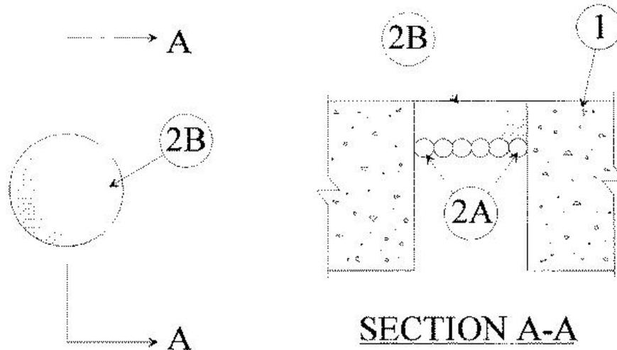
1. **Floor or Wall Assembly** — Min 4-1/2 in. thick reinforced lightweight or normal weight (100-150 pcf) concrete. Wall may also be constructed of any UL Classified **Concrete Blocks\***. Max diam of opening is 4 in. See **Concrete Blocks** (CAZT) category in the Fire Resistance Directory for names of manufacturers.
