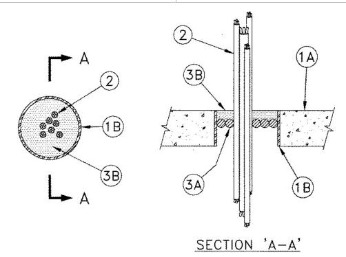
1A. **Floor or Wall Assembly** — Min 4-1/2 in. (114 mm) thick reinforced light weight or normal weight (100<u>150</u> pcf or 1600-2400 kg/m<sup>3</sup>) concrete. Wall may also be constructed of any UL Classified**Concrete Blocks**\*. Floor may also be constructed of any min 6 in. (152 mm) thick UL Classified hollow-core **Precast Concrete Units**\*. Max diam of opening is 6 in. (152 mm).
