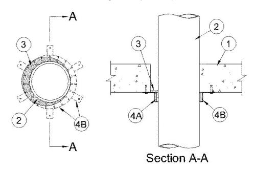
Floor or Wall Assembly — Min 4-1/2 in. (114 mm) thick reinforced lightweight or normal weight (100-150 pcf or 1600-2400 kg/m<sup>3</sup>) concrete. Wall may also be constructed of any UL Classified Concrete Blocks\*. Max diam of opening is 5 in. (127 mm). See Concrete Blocks (CAZT) category in the Fire Resistance Directory for names of manufacturers.
