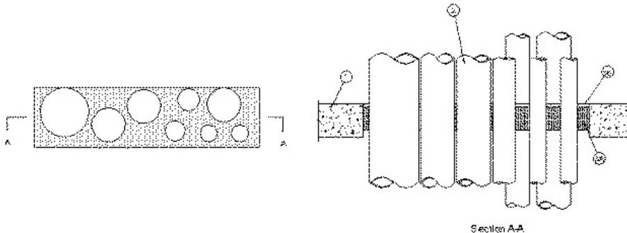
**1. Floor or Wall Assembly** — Min 4-1/2 in. (114 mm) thick reinforced lightweight or normal weight (100-150 pcf or 1600-2400 kg/m<sup>3</sup>) concrete floor. Wall may also be constructed of any UL classified **Concrete Blocks\***. Max area of opening is 240 sq in. (0.15 m<sup>2</sup>) with max dimension of 30 in. (762 mm).
