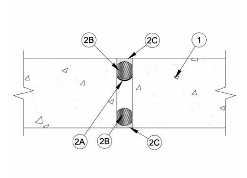
1. Wall Assembly — Min 6 in. (152mm) thick reinforced lightweight or normal weight (100<u>150</u> pcf or 1600-2400 kg/m³) structural concrete. Wall may also be constructed of any UL Classified **Concrete Blocks**\*.
