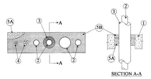
1. **Floor or Wall Assembly** — Min 4-1/2 in. (114 mm) thick reinforced lightweight or normal weight (100<u>150</u> pcf or 1600-2400 kg/m³) concrete floor or min 5 in. (1127 mm) thick reinforced lightweight or normal weight concrete wall. Wall may also be constructed of any UL Classified **Concrete Blocks\*.** Max area of opening is 144 sq in. (929 cm²) with max dimension of 24 in. (610 mm).
