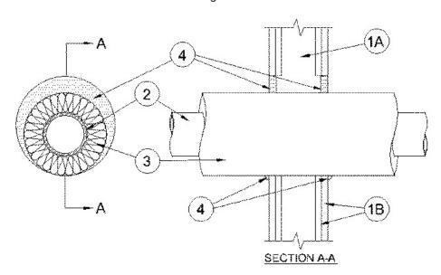
1. **Wall Assembly** — The 2 hr fire-rated gypsum board/steel stud wall assembly shall be constructed of the materials and in the manner specified in the individual U400 Series Wall and Partition Designs in the UL Fire Resistance Directory and shall include the following construction features:
