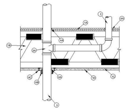
1. Floor-Ceiling Assembly — The 1 hr fire-rated solid or trussed lumber joist floor-ceiling assembly shall be constructed of the materials and in the manner specified in individual L500 Series Floor-Ceiling Designs in the UL Fire Resistance Directory, as summarized below:
