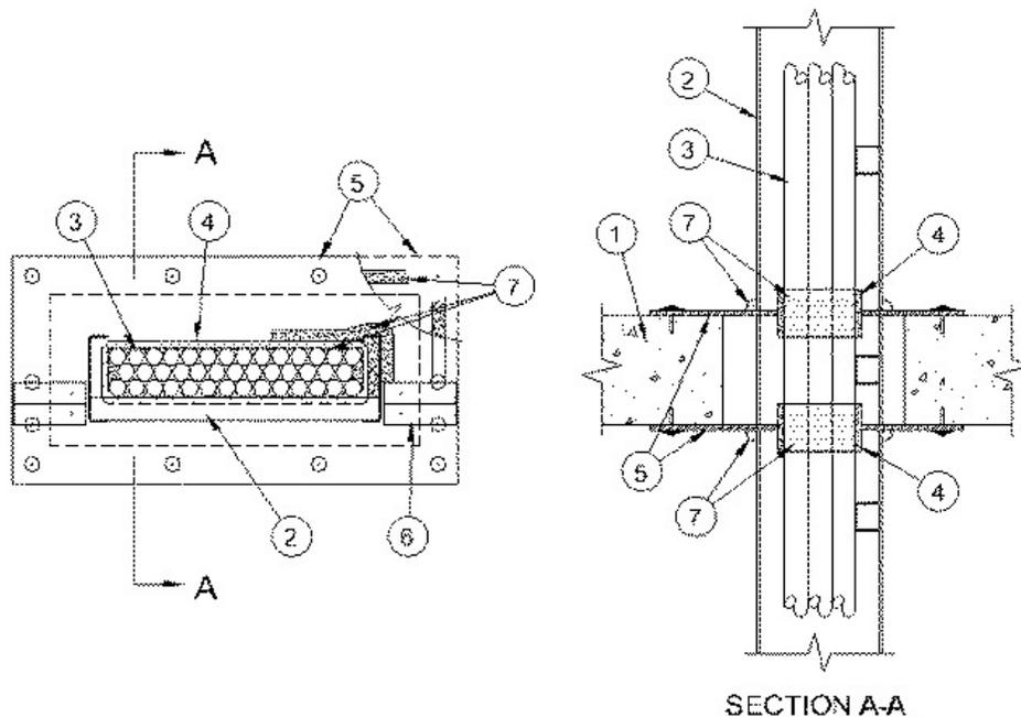
1. **Floor or Wall Assembly** — Min 4-1/2 in. (114 mm) thick lightweight or normal weight (100-150 pcf or 1600-2400 kg/m<sup>3</sup>) concrete. Wall may also be constructed of any UL Classified **Concrete Blocks\***. Max area of opening **900** sq in. (5806 cm<sup>2</sup>) with max dimension of 30 in. (762 mm).
