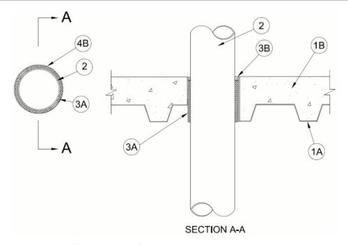
System tested with a pressure differential of 2.5 Pa between the exposed and the unexposed surfaces with the higher pressure on the exposed side.
