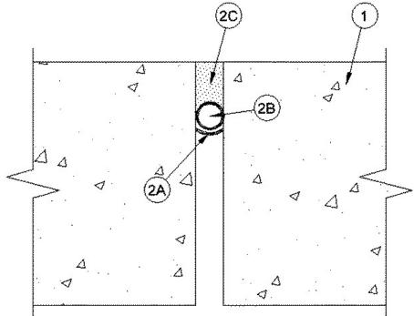
1. Floor Assembly — Min 4-1/2 in. thick reinforced lightweight or normal weight (100<u>150</u> pcf) structural concrete.
