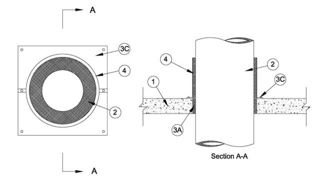
1. Floor or Wall Assembly — Min 4-1/2 in. (114 mm) thick reinforced lightweight or normal weight ( $100\frac{150}{100}$  pcf or 1600-2400 kg/m<sup>3</sup>) concrete. Wall may also be constructed of any UL Classified Concrete Blocks\*. Max area of opening is 13.75 f<sup>2</sup> (1.28 m<sup>2</sup>) with max dimensions of 44-1/2 in. (1.13 m).
