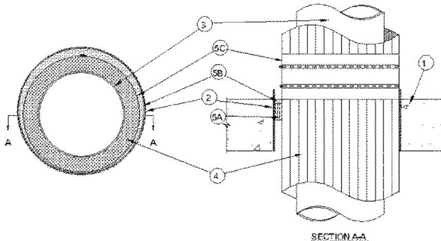
**1. Floor or Wall Assembly** — Min 4-1/2 in. thick reinforced lightweight or normal weight (100-150 pcf) concrete. Floor assembly may also be constructed of any min 6 in. thick UL Classified hollow-core **Precast Concrete Units\***. Wall may also be constructed of any UL Classified **Concrete Blocks\***. Max diam of opening 28 in. Max diam of opening in floors constructed of hollow-core concrete is 7 in.
