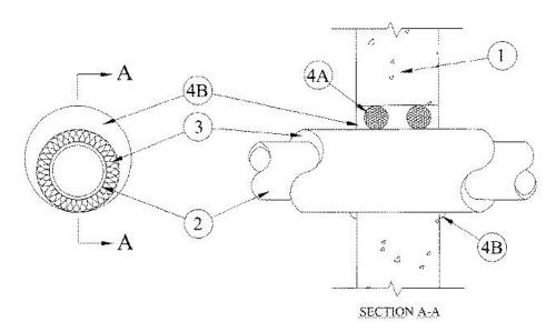
1. Wall Assembly — Min 6 in. thick lightweight or normal weight (100<u>150</u> pcf) concrete. Wall may also be constructed of any UL Classified Concrete Blocks\*. Max diam of opening is 8-1/2 in.
