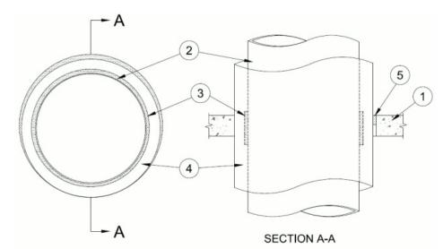
1. Floor or Wall Assembly — Min 4-1/2 in. (114 mm) thick lightweight or normal weight (100<u>150</u> pcf or 1600-2400 kg/ m<sup>3</sup>) concrete. Floor may also be constructed of any min 6 in. (152 mm) thick hollow-core **Precast Concrete Units**\*. Wall may also be constructed of any UL Classified Concrete Blocks\*. Max diam of opening to be 14-1/2 in. (368 mm). Max diam of opening in hollow-core precast concrete units is 7 in. (178 mm).
