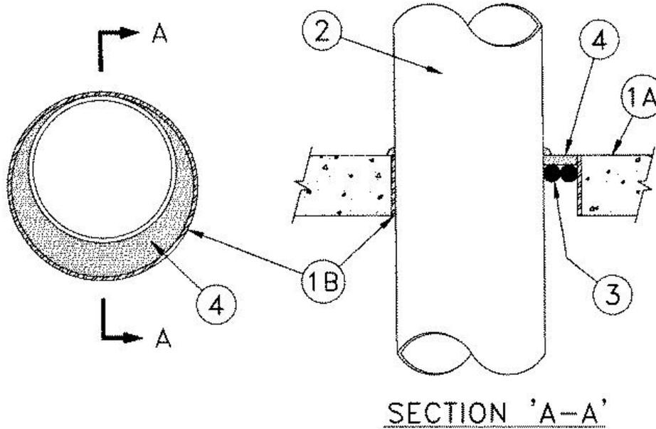
**1A. Floor or Wall Assembly** — Min 2-1/2 in. (64 mm) thick reinforced light weight or normal weight (100-150 pcf or 1600-2400 kg/m<sup>3</sup>) concrete. Floor may also be constructed of any min 6 in. thick UL Classified hollow-core precast units. Wall may also be constructed of any UL Classified **Concrete Blocks**\*. Max diam of opening is 10-3/4 in. (273 mm).
