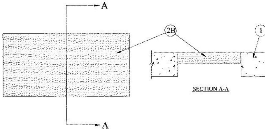
**1. Floor or Wall Assembly** — Min 4-1/2 in. thick reinforced lightweight or normal weight (100-150 pcf) concrete. Wall may also be constructed of any UL Classified **Concrete Blocks\***. Max area of opening is 288 sq in. with max dimension of 24 in.
