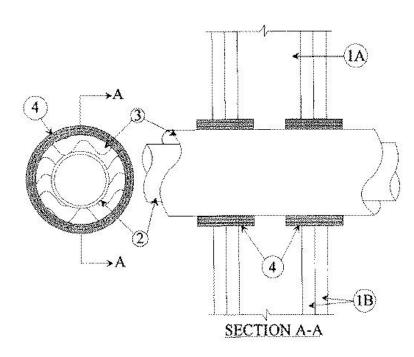
1. **Wall Assembly** — The fire-rated gypsum wallboard/stud wall assembly shall be constructed of the materials and in the manner specified in the individual U300 or U400 Series Wall and Partition Designs in the UL Fire Resistance Directory and shall include the following construction features:
