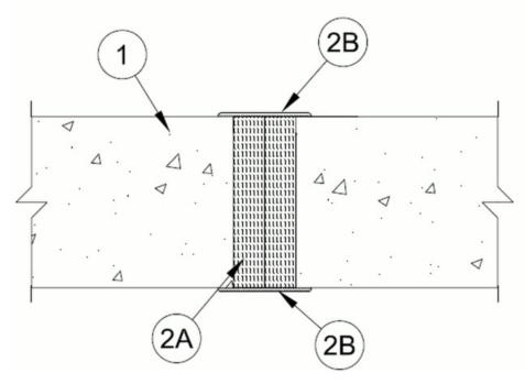
Wall Assembly — Min 5-7/8 in. (149 mm) thick reinforced lightweight or normal weight (100<u>150</u> pcf or 1600-2400 kg/m<sup>3</sup>) structural concrete. Min 3 hr fire rated U900 Series wall may also be constructed of UL Classified Concrete Blocks\*. See Concrete Blocks (CAZT) category in the Fire Resistance Directory for names of manufacturers.
