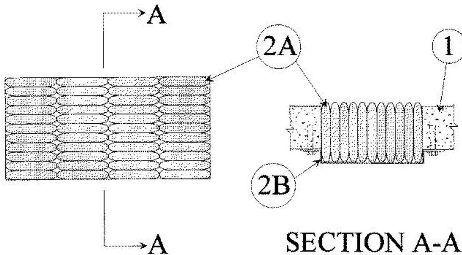
1. **Floor or Wall Assembly** — Min 4-1/2 in. thick reinforced lightweight or normal weight (100-150 pcf) concrete. Max area of opening is 288 in. with max dimension of 24 in.
