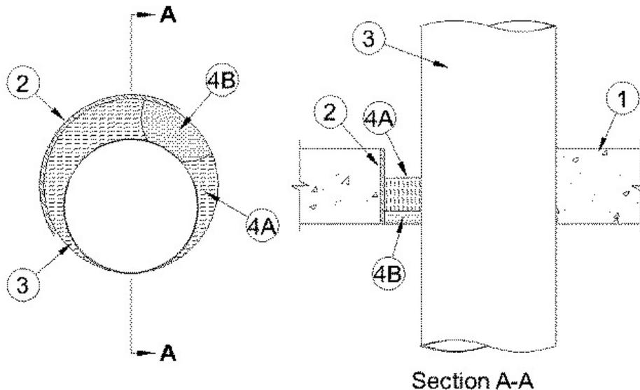
**1. Floor or Wall Assembly** — Min 4-1/2 in. (114 mm) thick reinforced lightweight or normal weight (100-150 pcf or 1600-2400 kg/m<sup>3</sup>) concrete. Floor may also be constructed of any min 6 in. (152 mm) thick UL Classified hollow core **Precast Concrete Units\***. When precast concrete units are used, the max diam of opening is 7 in. (178 mm). Wall may also be constructed of any UL Classified **Concrete Blocks\***. Max diam of opening is 8-1/2 in. (216 mm).
