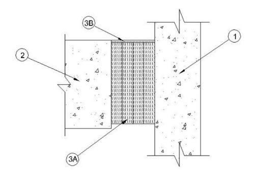
1. **Wall Assembly** — Min 4-1/2 in. (114 mm) thick steel-reinforced lightweight or normal weight (100<u>150</u> pcf or 1600-2400 kg/m<sup>3</sup>) structural concrete. Wall may also be constructed of any UL Classified **Concrete Blocks**\*.
