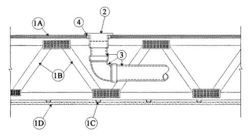
1. Floor-Ceiling Assembly — The 1 hr fire-rated solid or trussed lumber joist floor-ceiling assembly shall be constructed of the materials and in the manner specified in individual L500 Series Floor-Ceiling Designs in the UL Fire Resistance Directory, as summarized below:
