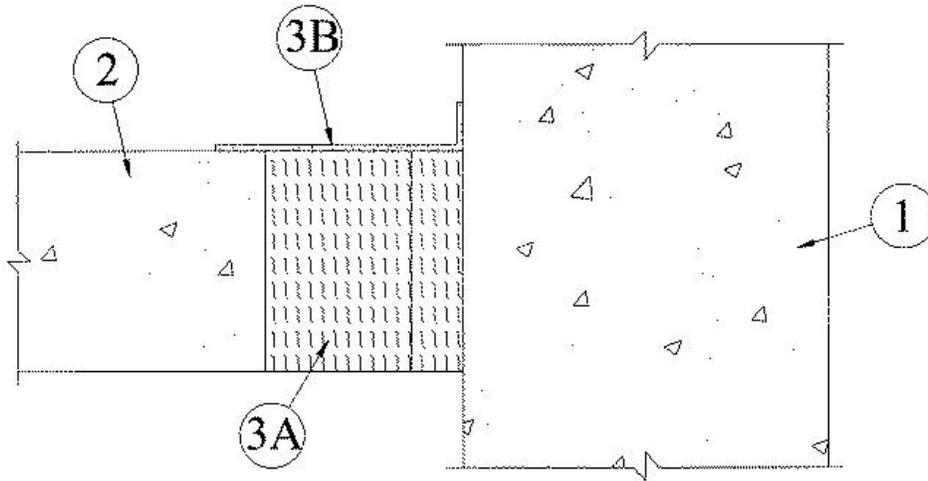
**1. Wall Assembly** — Min 7-3/8 in. (187 mm) thick reinforced lightweight or normal weight (100-150 pcf or 1600-2400 kg/m<sup>3</sup>) structural concrete. Wall may also be constructed of any UL Classified **Concrete Blocks\***.
