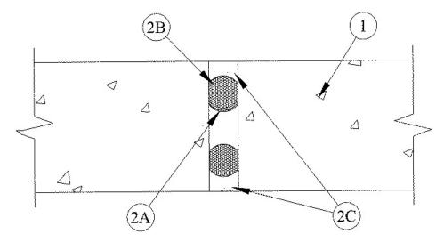
1. **Wall Assembly** — Min 4-1/2 in. thick reinforced lightweight or normal weight (100<u>150</u> pcf) structural concrete. Wall may also be constructed of any UL Classified **Concrete Blocks**\*.
