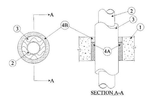
1. Floor or Wall Assembly — Min 4-1/2 in. thick reinforced lightweight or normal weight (100<u>150</u> pcf) concrete floor or min 5-1/4 in. thick reinforced lightweight or normal weight concrete wall. Wall may also be constructed of any UL Classified **Concrete Blocks\*.** Max diam of opening is 4 in.
