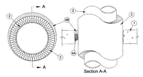
1. Floor or Wall Assembly — Min 4-1/2 in. thick reinforced lightweight or normal weight (100<u>150</u> pcf) concrete. Wall may also be constructed of any UL Classified Concrete Blocks\*. Floor may also be constructed of any 6 in. thick UL Classified hollow-core **Precast Concrete Units**\*. Max diam of opening is 16 in. When precast conrete units are use, max diam of opening is 7 in.
