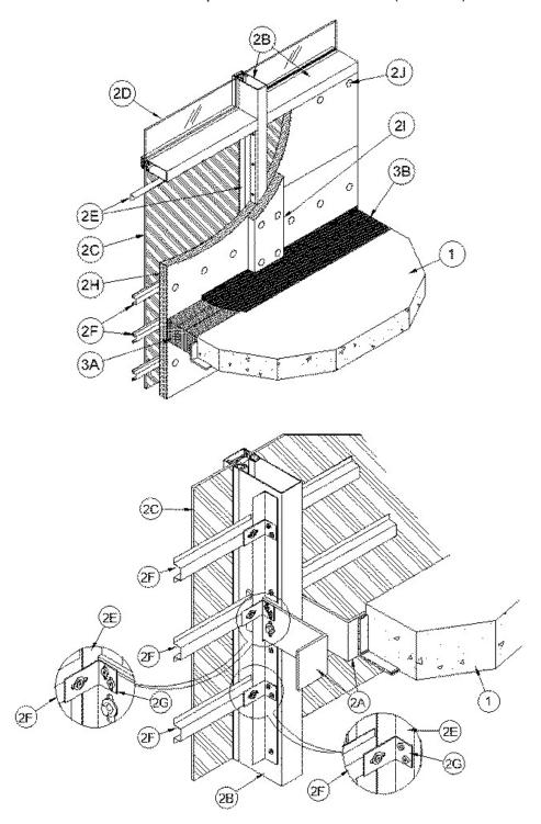
1. Floor Assembly — Min 4-1/2 in. thick reinforced lightweight or normal weight (100<u>150</u> pcf) structural concrete. Perimeter of floor assembly to be provided with min 4 by 4 by 1/4 in. thick cast-in-place structural steel angle for weld-attachment of mullion mounting clips (Item 2A).
