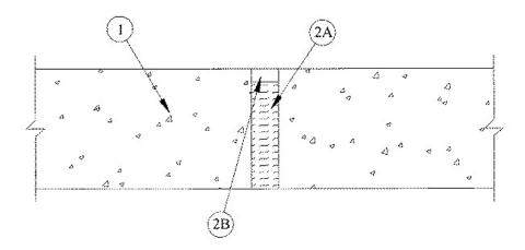
1. Floor Assembly — Precast Autoclaved Aerated Concrete\* — Min 4 in. (102 mm) thick as specified in Design No. K909, K910, P932 or P933 in the UL Fire Resistance Directory.
