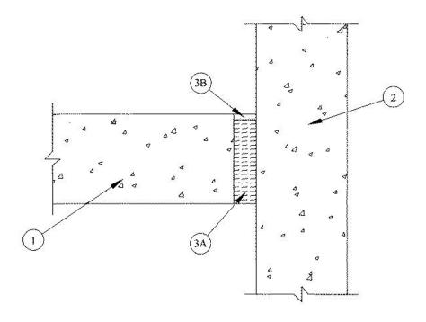
1. Floor Assembly — Precast Autoclaved Aerated Concrete\* — Min 4 in. (102 mm) thick as specified in Design No. K909, K910, P932 or P933 in the UL Fire Resistance Directory.
